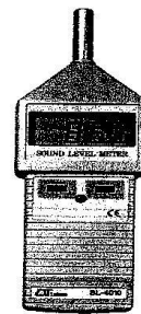
Figure (4): Pre-Calibrated Sound Level Meter At 114 dB(A)
